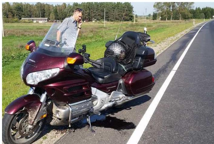
**Gary's Gold Wing was disabled after hitting a large bolt that punctured his engine casing.**
